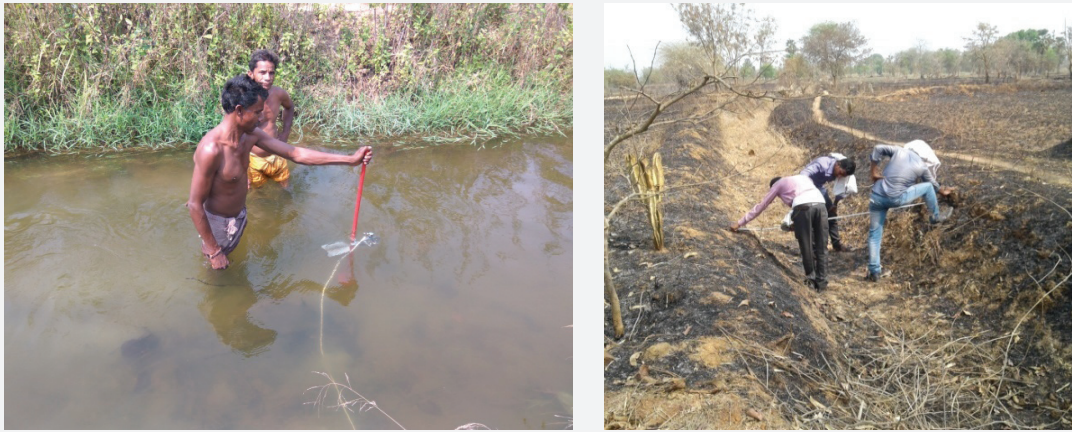
FIGURE 32: (A) Measurement water velocity with Cup type current meter in a minor of Hariharjore medium project; (b) Measurement of actual cross section of Sakma Minor of Bhimtikira distributary, Hirakud Major Project
